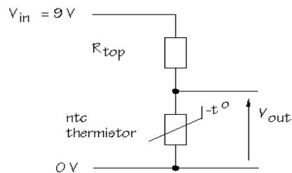
Fig. 4. Circuit diagram of NTC Thermistor
