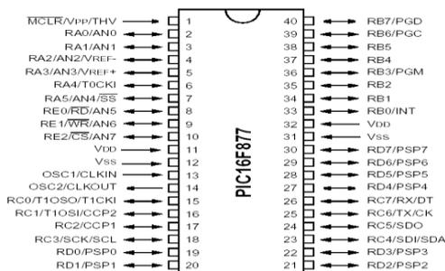
Fig. 1. Pin diagram of PIC 16F877A
