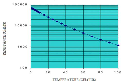
Fig. 5. Thermistor Characteristic Curve
